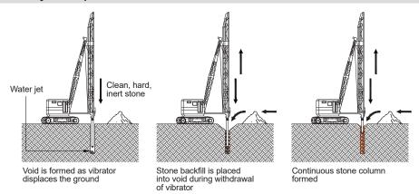
Where the ground contains fines and silts, water jetting from the tip of the vibroflot is used to remove loose materials and form a cavity for charges of stone to be added to replace and densify the soft ground. The carbon footprint of this activity is generally less than with comparable piling solutions.
