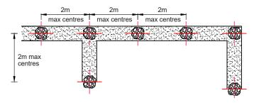
Stone columns which are misaligned by more than 150mm (centre to centre) in any direction should be replaced.
